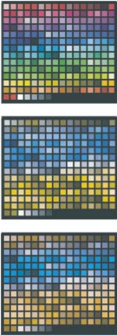
Figure 12. Top: The Websafe palette of 216 colours. Middle: Transformation of the Websafe palette to the colours perceived by deuteranopes. Bottom: Transformation of the Websafe palette to the colours perceived by protanopes. © 2004 British Telecommunications plc. Reproduced with permission.
